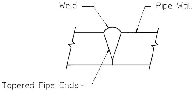
FIG. 4 Extrusion Weld
