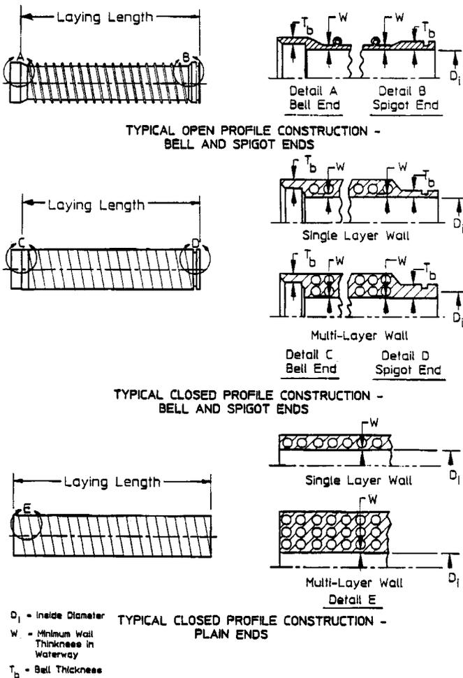
FIG. 1 Typical Construction of Profile Wall PE Pipe
